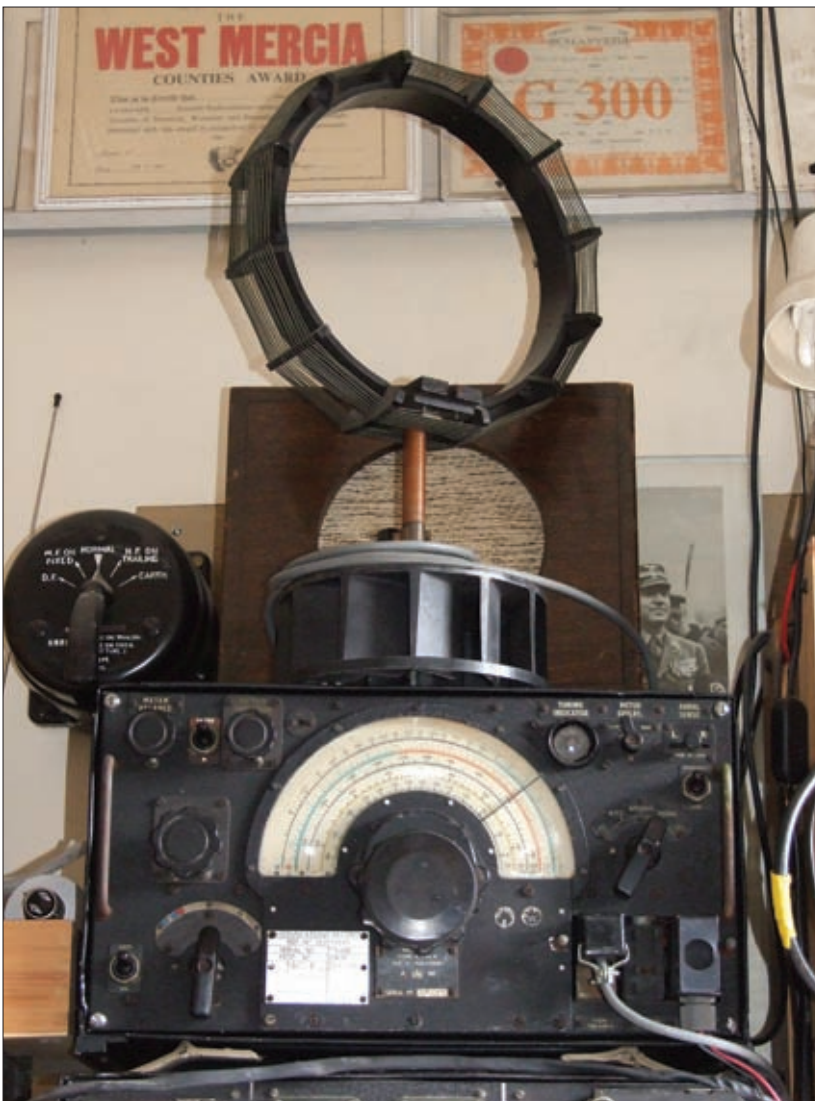
Fig 1: The R1155 receiver and its loop antenna.
